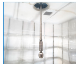
Spray assembly shown mounted inside IBC tote, with Alfa Laval MultiMidget device.
